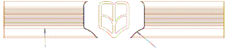
The contour fit at cross intersection. Note, the absence of the side ridges on the primary seal to assure a tight flat contact.
