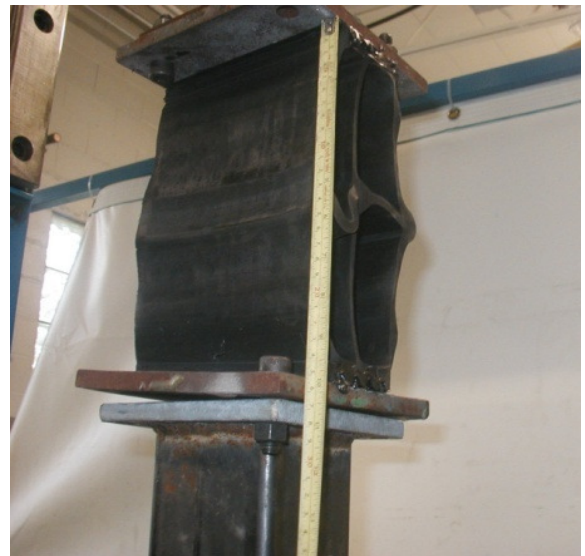
Extreme tension testing of JP-400 (4 inch) expansion joint system to almost 13 inches.
