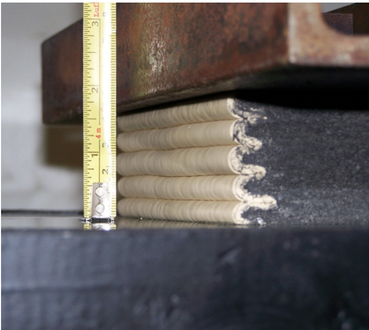
Compression testing of pre-compressed foam seal against window glass to assure that the glass and seal will not be affected
